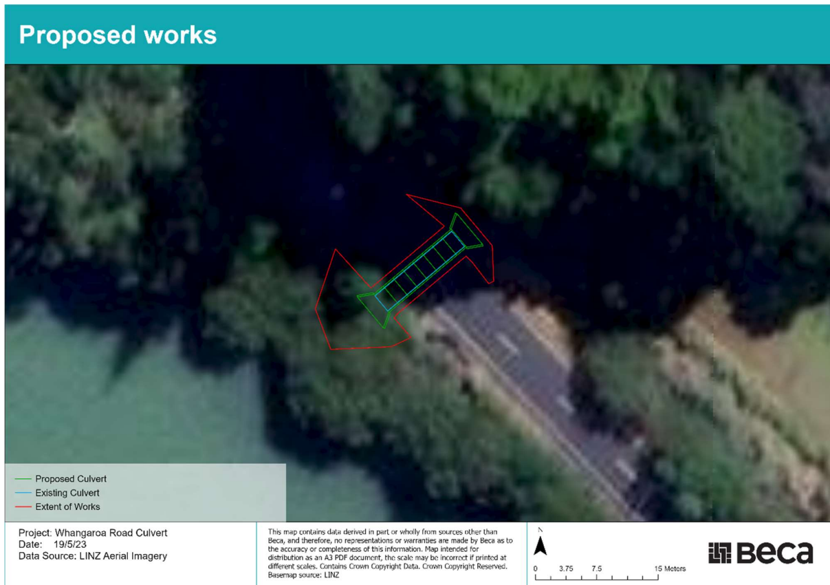
Figure 3.1. Indicative area of the proposed works overlaying an aerial photo of the site. The proposed structure is shown in green and blue with the extent of the earthworks and disturbance in red.
